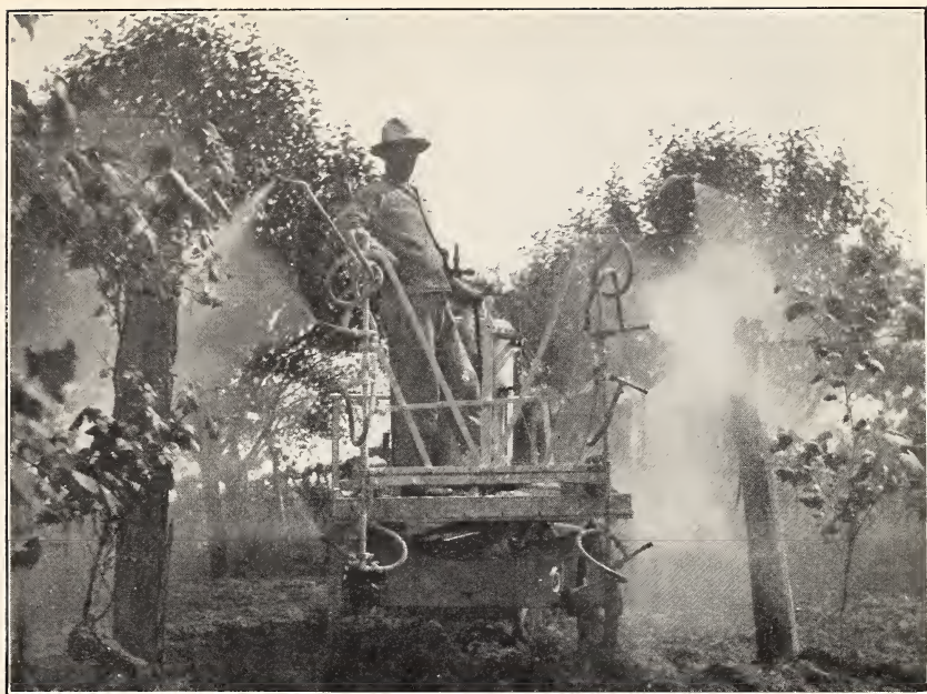
FIG. 1.—CARBONIC-ACID-GAS SPRAYER USED IN SPRAYING EXPERIMENTS IN 1907 AND 1908 IN THE VINEYARD OF MRS. EMMA R. SMITH, PAW PAW, MICH.
